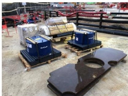
Figure 5. Instrumentation used for a designed 70 MN load test in a barrette (Fugro).
