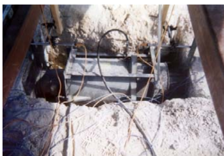
Conventional lateral load test
