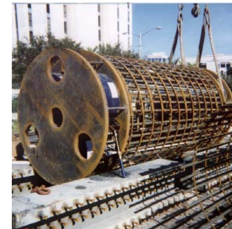
High capacity testing with multiple O-cells
