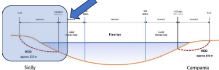
Figure 5 - Contractual cables burial scheme for HVDC cables
