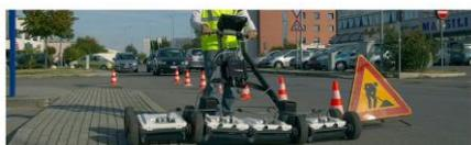
A specialised ground penetrating radar (GPR) system, RIS MF Hi-Mod is capable of investigating large areas, providing a 3D view of the subsoil with a high capability of resolution and penetration depth. RIS MF Hi-Mod features:
