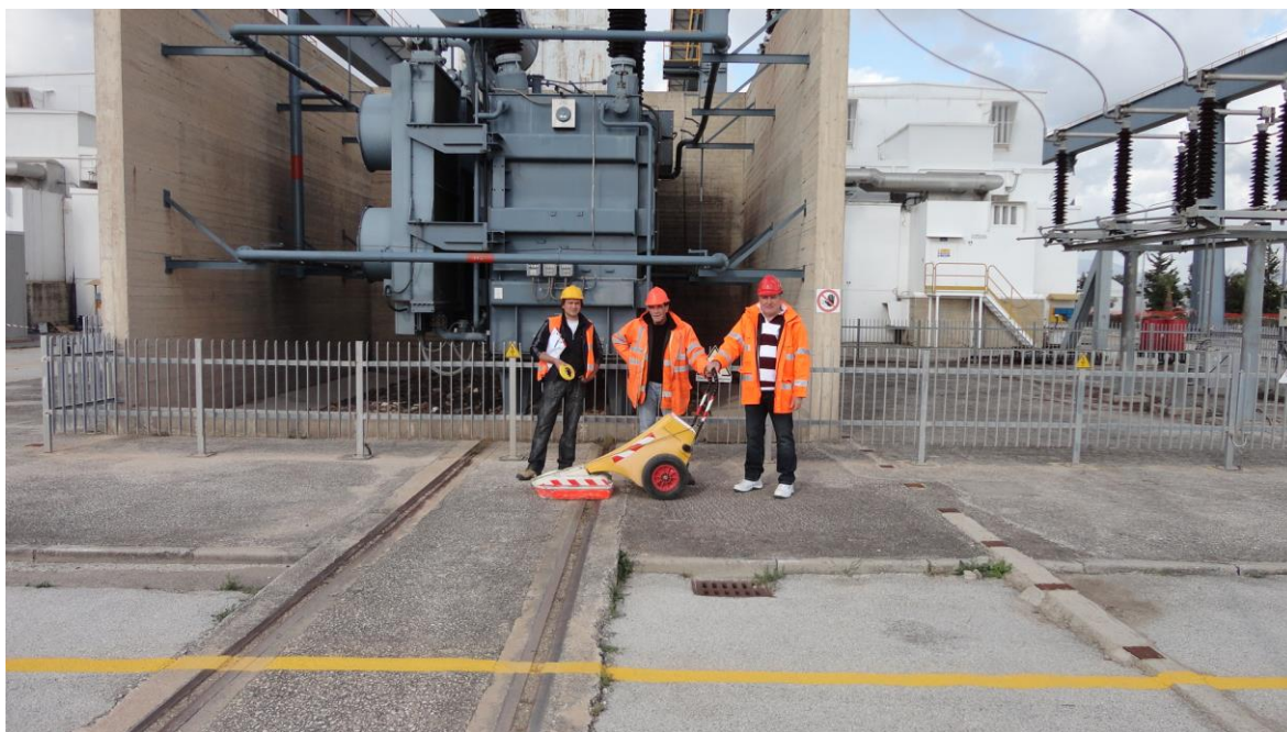
SCANGEA performing a GPR survey at the E.ON Power Plant in Trapani (April 2012).
